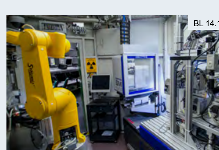
Beamline 14.1 • Energy range 5.5 – 19.5 keV • 5.0 \times 10^{11} photons/s • High performance multi-axis goniometer MD2 • Automated sample mounting • PILATUS 6M detector • High performance de novo structure determination by MAD/SAD
